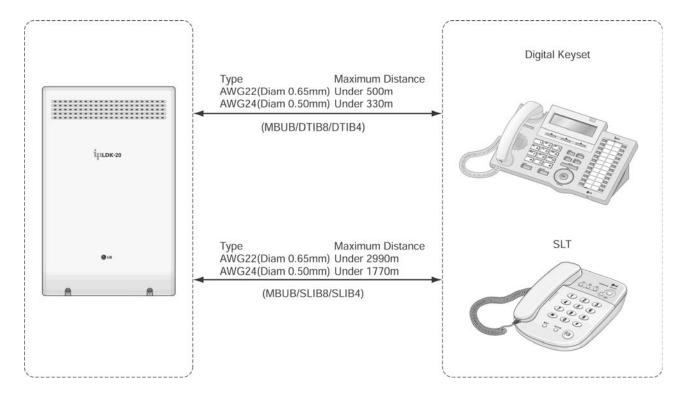
Figure 5.2 Terminal Cabling Distance
